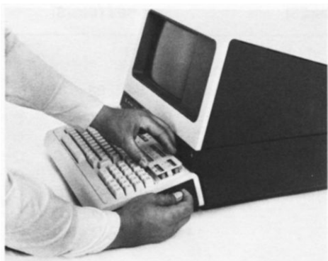
A. REMOVING A KEYBOARD OVERLAY
