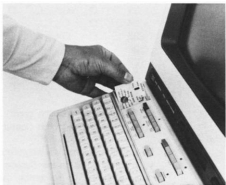
B. INSTALLING BAUDRATE OVERLAY
